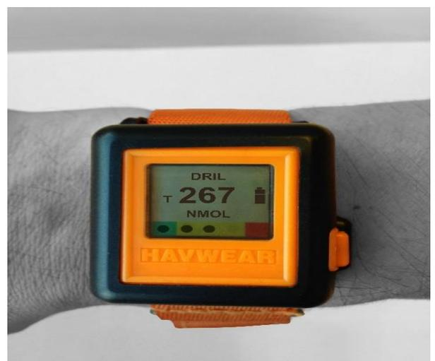
Figure 1 Reactec wearable HAVS monitor
